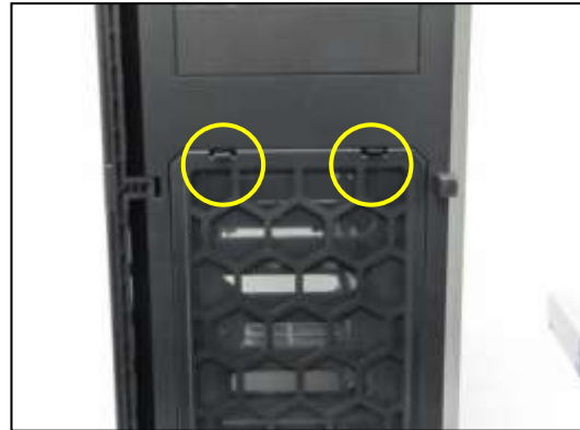
Open the front door by pushing down on the tabs (circled above) at the top of the front filter.
