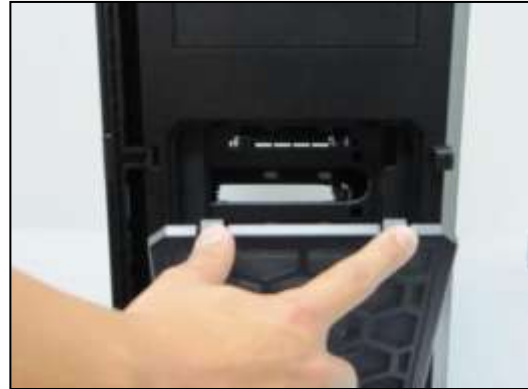
Open the front door by pushing down on the tabs (circled above) at the top of the front filter.
