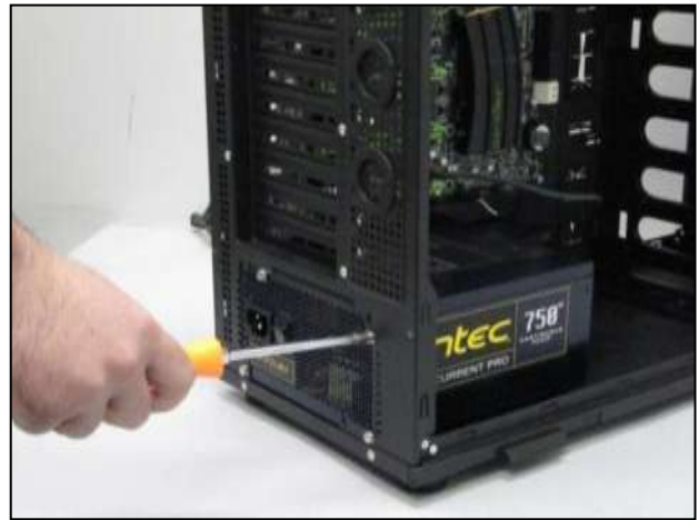
Attach the power supply with the provided screws.
