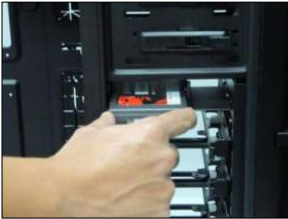
Slide your 2.5" drive into the drive bay so that the drive's holes align with the drive bay holes.
