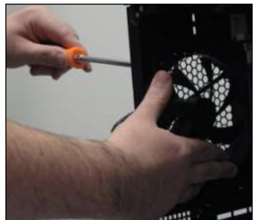
Unscrew the rear fan to remove it.
