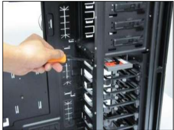
Secure your drive with the provided 2.5" screws.
